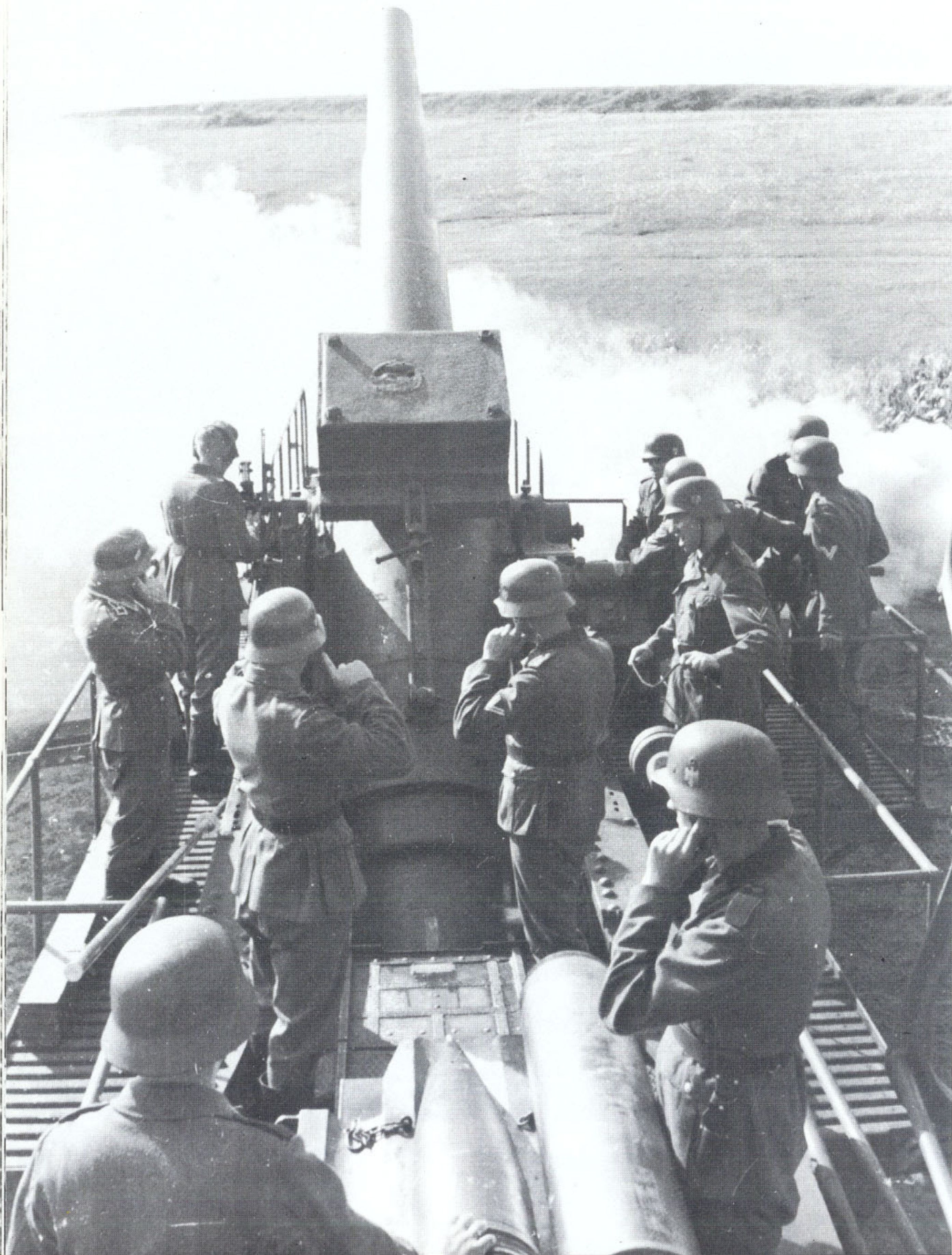
A view of the gun just after the weapon has been fired—note the cloud of dust in front of the gun, raised by the muzzle blast. Next the barrel will be lowered to the horizontal “loading” position and the shell and propellant charge on the loading cradle will be pushed into the breech for the next shot.
