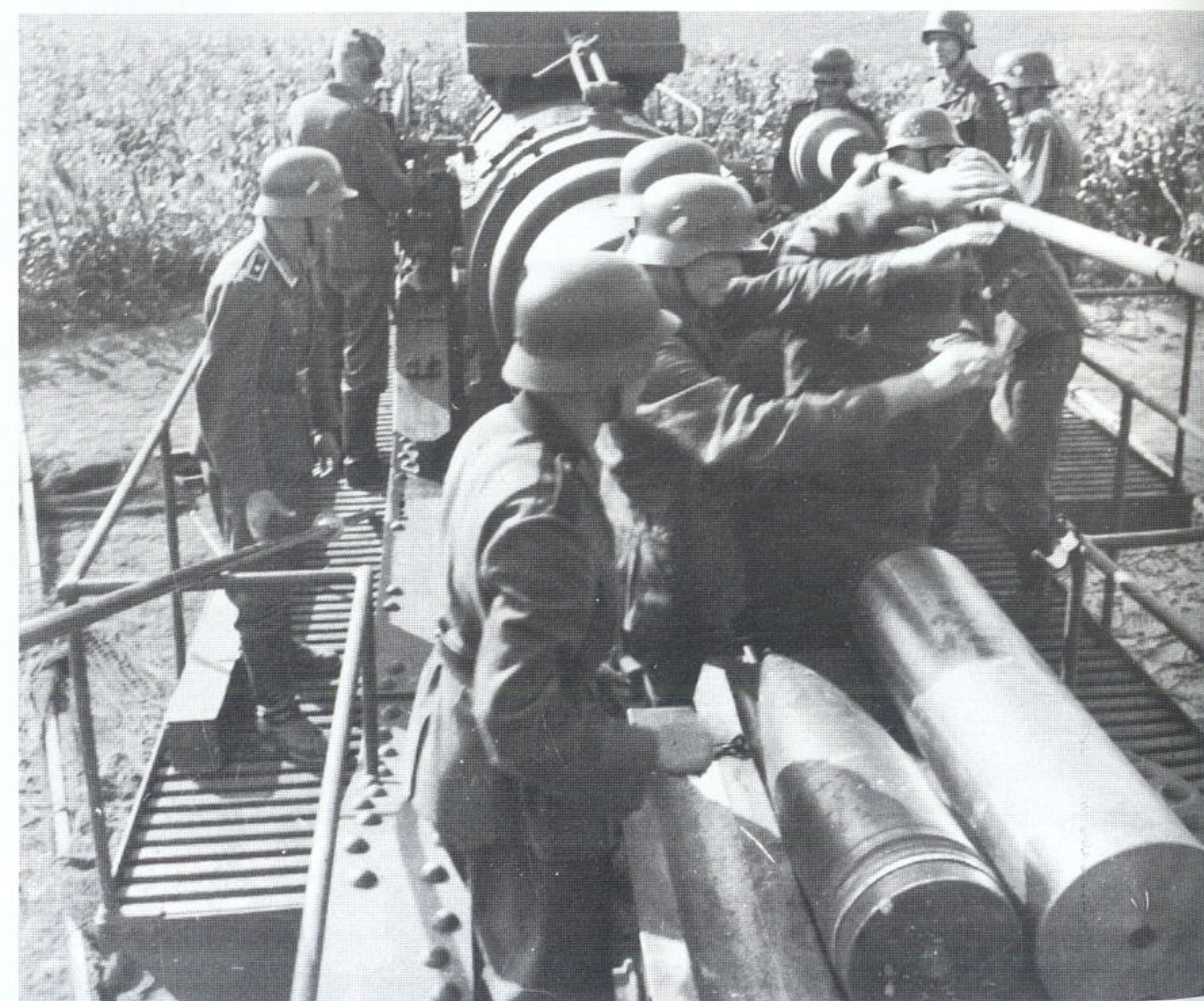
The loading ramrod is passed aside prior to closing the breech. Shown is a rear view of the loading cradle with the next shell and case. The barrel was lowered to the horizontal "loading" position after each shot, as all loading operations had to be conducted with barrel horizontal.
