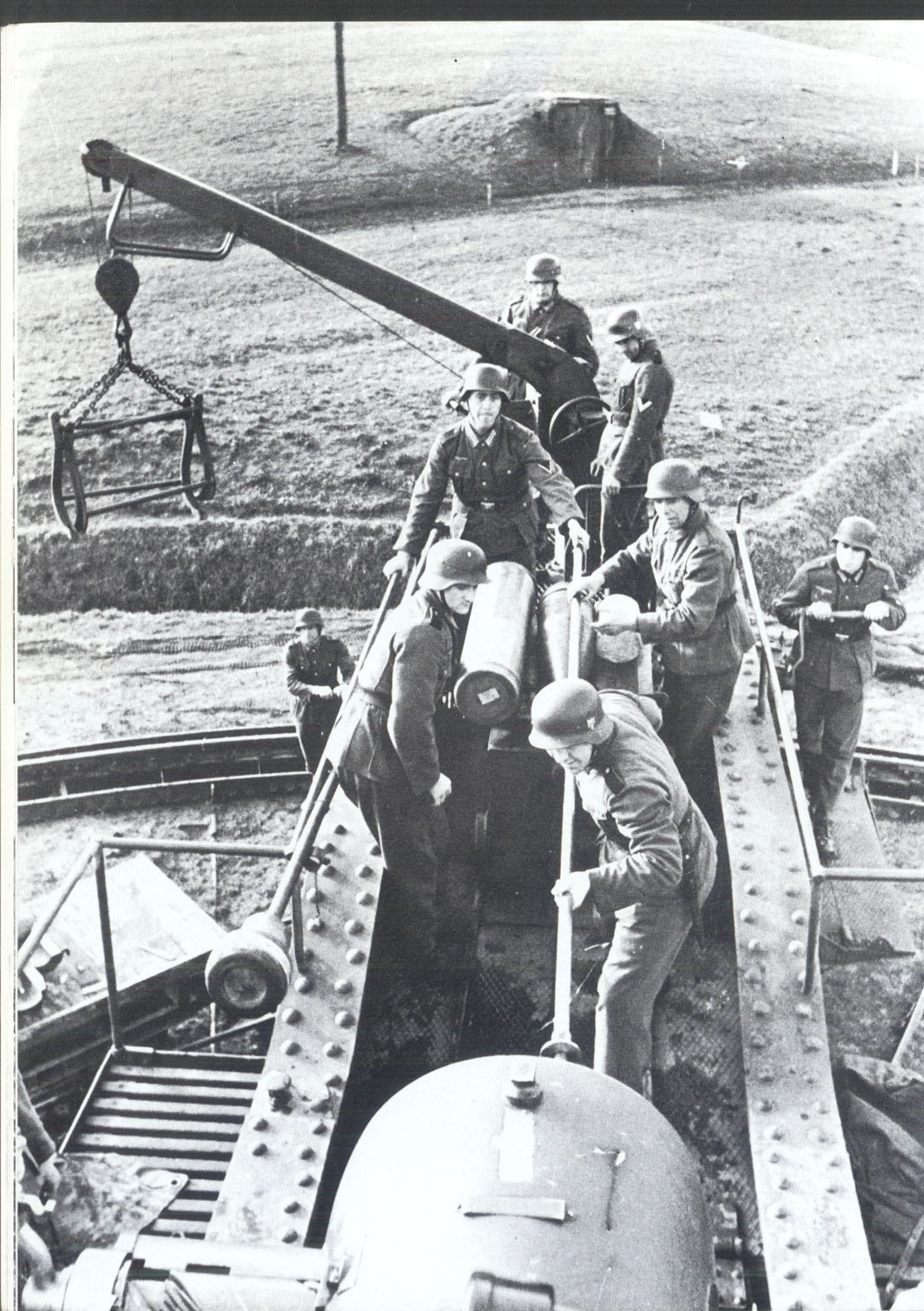
Here the gun crew rams the propellant casing into the breech prior to firing. Note the second shell and propellant case on the loading cradle, ready to be loaded for the following shot.
